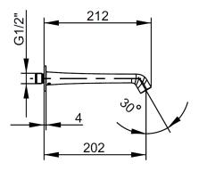
Note: Spout comes with a 1/2" male thread. 1/2" female outlet required in the wall
